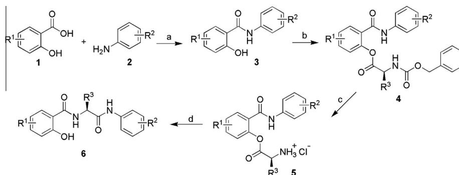
**Scheme 1.** Synthesis of 2-hydroxy-*N*-[(2*S*)-1-oxo-1-(phenylamino)alk-2-yl]benzamides. Reagents and conditions: (a)  $\text{PCl}_3$ , PhCl, MW, 400 W, 20 min; (b) DCC, DMF,  $-10^\circ\text{C}$ , 2 h; *N*-Cbz-AA (c) 33% HBr/AcOH, RT, 30 min; (d) TEA,  $\text{CHCl}_3$ , RT, 30 min.
